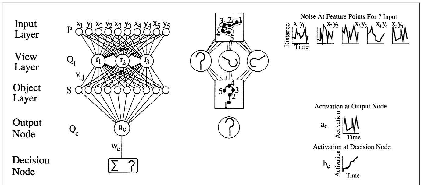
**Fig. 2.** A Poggio-Edelman module that recognizes question marks. The left side depicts the nodes of the module, the center gives a schematic of what the nodes represent, and the right side shows input and activation values over time.
