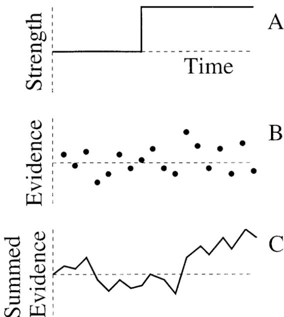
**FIG. 2.** An induction from a stepped stimulus (Panel A) to an evidence stochastic process (Panel B). Panel C shows the summation of evidence as specified by a random walk. Once the evidence stochastic process is realized (Panel B), the random walk summation shown in Panel C is deterministic.
