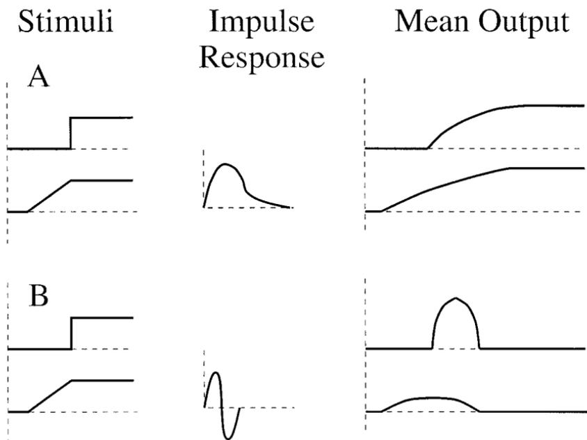
**FIG. 3.** Monotonic and nonmonotonic inductions. Panel A shows the case for a linear filter with a nonnegative impulse response function. The output for ramped stimuli dominates that for stepped stimuli. If the impulse response violates nonnegativity, the output from stepped stimuli may not dominate that from ramped stimuli, as depicted in Panel B.
